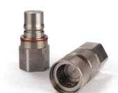
The NSE are dry-break couplings with flat face valves. The compact design makes it suitable for reduced spaces when high flow is needed. Coupling system with two-hand operation, i.e. both hands are required when connect/disconnect.
