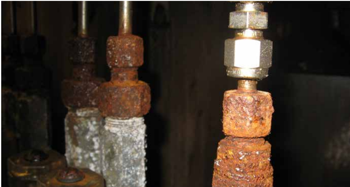
Galvanic reaction created by mixing different body & nut materials.
