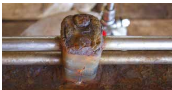
Crevice corrosion between the tube/tube trap interface.
