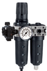
Slide Valve + Filter/Regulator + Lubricator Combinations (50mg/m 3 ) 5 micron element, 8 bar Regulator + Gauge and Wall Mounting Brackets
