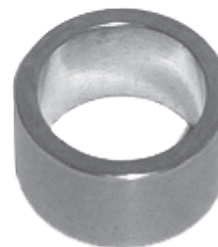
As-machined + Suparcase® Test Piece After Ferric Chloride Test
