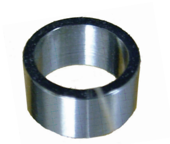
As-machined + Suparcase® Test Piece After Salt Fog Test
