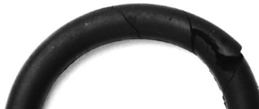
Fig. 10.10 Twisted O-Ring with cuts in surface
