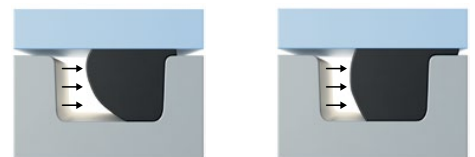
Fig. 10.3 At higher pressure a larger O-ring volume is pushed into the gap. A back-up ring prevents gap extrusion.
