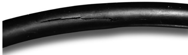
Fig. 10.11 O-Ring damaged by explosive decompression
