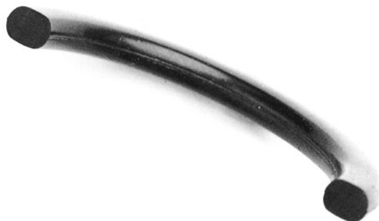
Fig. 10.8 Damage pattern caused by high compression set
