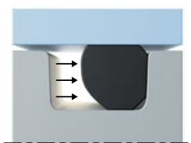
Fig. 10.2 On pressurising, the O-Ring acts like an incompressible fluid, exerting a pressure on the gland proportional to the system pressure
