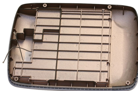
Plastic electronics housing painted with electrically conductive copper-filled coating
