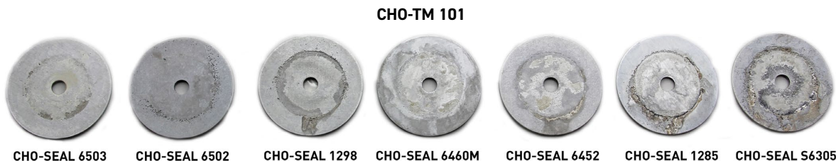
Figure 2-2: Picture of Corrosion Coupon After 504 salt spray/salt fog
