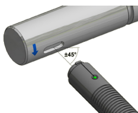
Rotating shaft: Contactless speed measurement.
