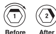
4. After hand tight, turn element clock wise 60° (or movement equal to one hex flat).
