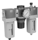
Filter + Regulator + Lubricator Combinations, poly bowl 5 micron element, 116 psig (8 bar) regulator + gauge and wall mounting brackets
