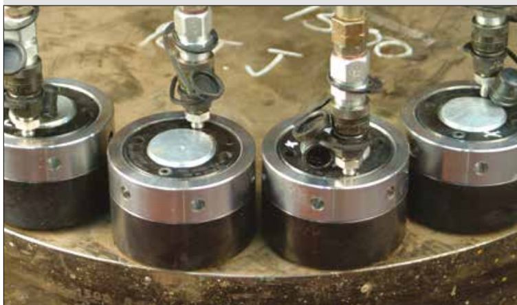
▲ Tensioning with hydraulic nuts.
