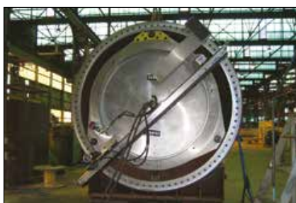
▼ Wind tower machining with WP4600.
