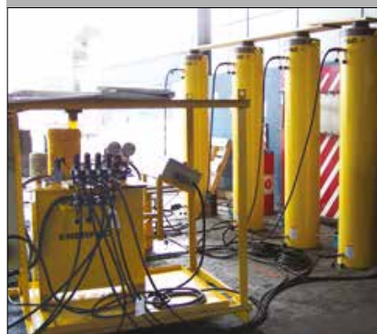
▲ Custom 500 ton double-acting cylinders with 1,83 m stroke for lifting electric rope shovels.
