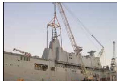
Synchronous hoisting and load positioning
