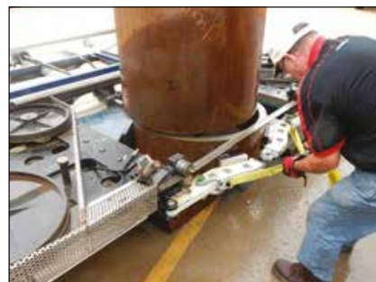
▲ Pipe cutting with BS portable band saw.
