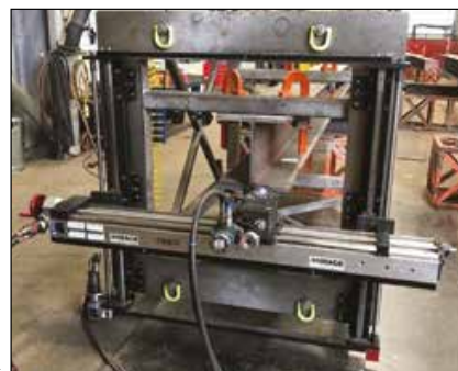
I-Beam end face milling with a GMRF1000. ►
