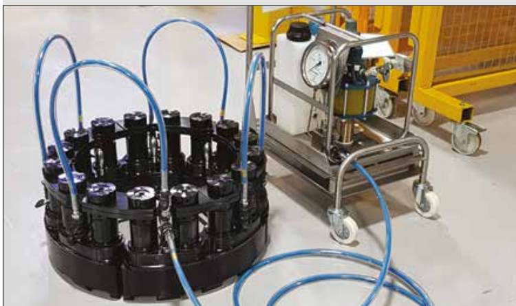
▲ Multi Stud Tensioning Set-Up.
