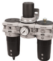
Combination Filter + Regulator + Lubricator, 12 bar, 5 micron
