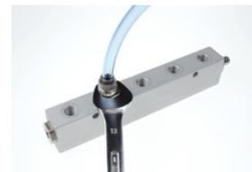
Tighten the nut by hand (in the case of soft tubing) or using a spanner (for semi-rigid tubing) until it comes into contact with the end stop.
