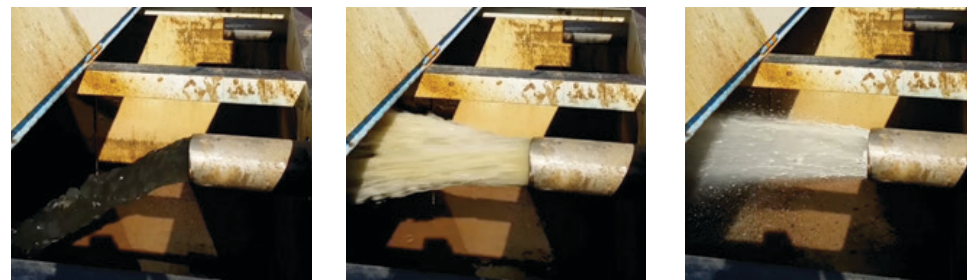
The pictures above show the backflush cleaning process of the BlastPure system. The dirty, contaminated water is literally blasted off the metallic filter cartridges during the cleaning cycle. The water color coming out from the blast goes from dark to clear as the filter cartridges are cleaned and prepared to be put back online.
