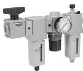
Ball Valve + Filter + Regulator + Lubricator Combinations, poly bowl 5 micron element, 116 psig (8 bar) regulator + gauge and wall mounting brackets
