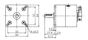
$\textbf{Note}: A \ \text{foot plate} \ \text{can} \ \text{be} \ \text{fitted} \ \text{turned} \ \text{by steps} \ \text{of} \ 60^{\circ} \ \text{from the original position}$
