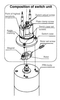
Mount the switch unit on the body using the set of screws. For clamping torque, refer to the table below
