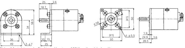
$\textbf{Note}: A \text{ foot plate can be fitted turned by steps of } 90^{\circ} \text{ from the original position}$
