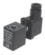
This miniature coil is designed for valves equipped with a miniature tube assembly. This is an encapsulated assembly comprising a coil, integral magnetic iron path and snap-on plug connection. The synthetic material encapsulation provides an effective compact housing, offering full protection against dust, oil, water, etc. Ease of mounting in confined space - offers shock and corrosion protection - simplifies conversion of existing equipment to other requirements, etc.
