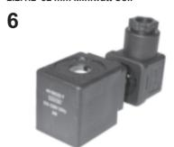
This reduced power coil is compatible with certain types of Lucifer solenoid valves only. This is an encapsulated assembly comprising a coil, integral magnetic iron path and snap-on plug connection. The synthetic material encapsulation provides an effective compact housing, offering full protection against dust, oil, water, etc. Ease of mounting in confined space - offers shock and corrosion protection - simplifies conversion of existing equipment to other requirements, etc.
