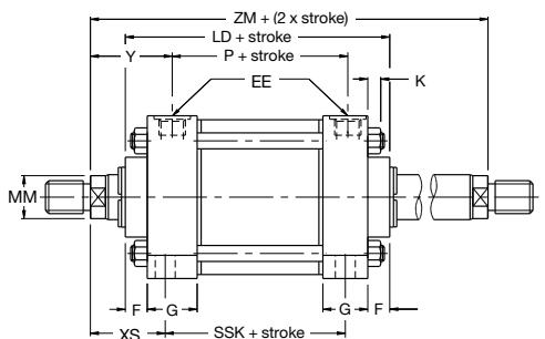
**Double Rod Cylinders – 203.2 to 355.6mm Bore Sizes**
