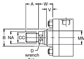
**Rod End Style 9**
