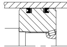
**Non-Lubricated Pistons** – For non-lubricated air cylinders, lipseals with special rounded sealing lips are supplied as standard. Specify Series 2AN (see pages 34-35).
