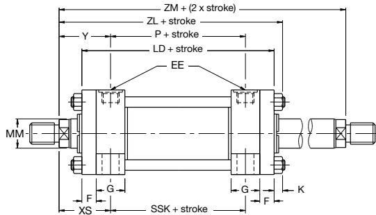
**Double Rod Cylinders – 25.4 to 152.4mm Bore Sizes**
