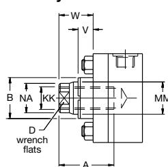
**Rod End Dimensions – 25.4mm to 152.4mm (1" to 6") bore sizes**
