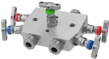
Example shown: 5-valve remote/line mount manifold featuring the Parker A-LOK® Superior Advantage Inverted integral tube fitting connections for the impulse line and NPT ported connections for the vent/ drains.
