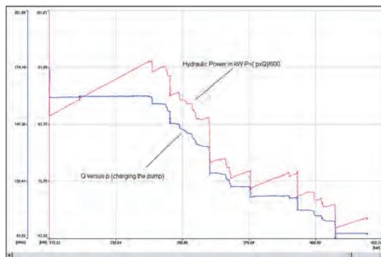
Combined pressure and volume flow measurement (figure on the left) allows insights into a system's hydraulic performance.
