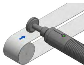
Contact speed measurement with contact adapter.
