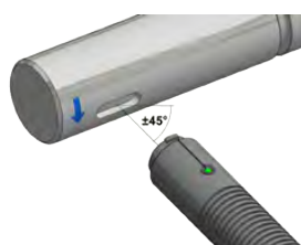
Rotating shaft: Contactless speed measurement.
