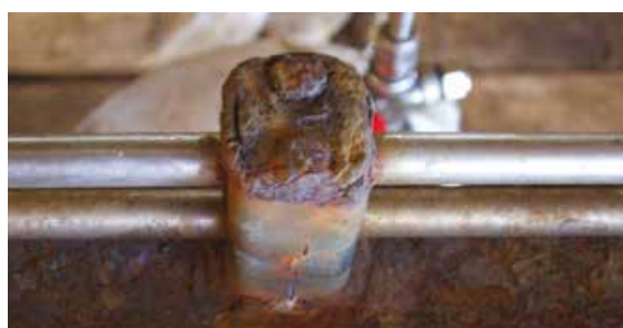
Crevice corrosion between the tube/tube trap interface.
