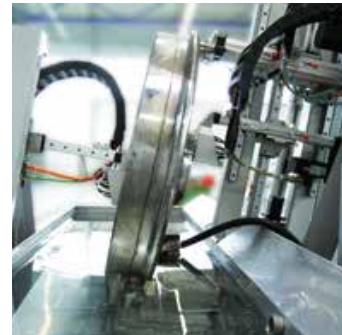
5 Deburring of Alloy Wheels Vertical and horizontal movement of sawing units
