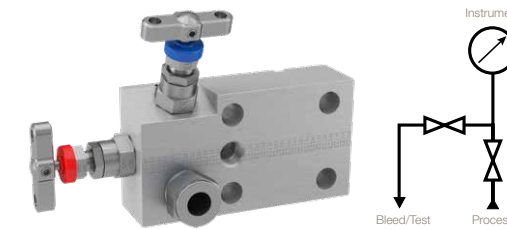
Example shown: 2-valve manifold with inverted integral A-LOK® connections.
