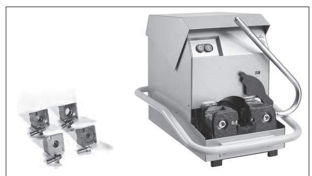
The Parflange® 1025 machine is designed to cold-form high pressure tube connections for O-Lok® and Triple-Lok® connection. It uses the Parflange® orbital flaring process. The Parflange® 1025 machine smoothly compresses the tube material and achieves a high strength joint with a polished surface of the tube end. O-Lok® and SAE flange sleeves are firmly fixed onto the tube end, resulting in a very rigid highpressure tube connection.
