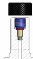
Model of valve stem integrated 5/8" 18 UNF (D)
