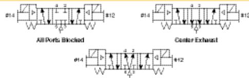
*With #12 operator energized* – inlet port 1 connected to cylinder port 2, cylinder port 4 connected to exhaust port 5.
