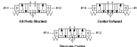
*With #12 operator signaled* – inlet port 1 connected to cylinder port 2, cylinder port 4 connected to exhaust port 5.
