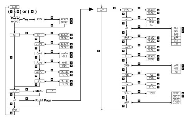
To Program Outputs and Options of SCPSD, press and hold the ▲ (Up Arrow Icon) then press the ▲ (Circle Icon) until Pro6 is displayed. Release all buttons and follow menu to program outputs and options.
