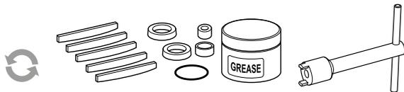
The first service is due after approximately 500 hours of operation. After the first service, the service interval is determined by the degree of vane wear.
