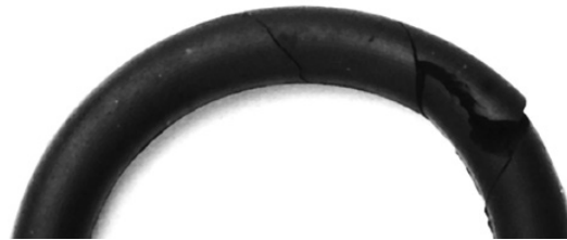
Fig. 10.10 Twisted O-ring with cuts in surface
