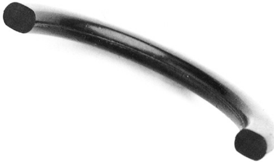
Fig. 10.8 Damage pattern caused by high compression set
