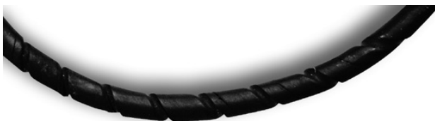
Fig. 10.9 Twisted O-ring with spiral markings
