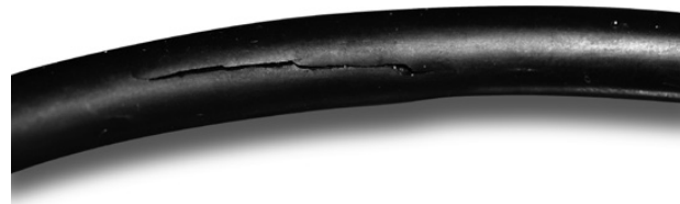
Fig. 10.11 O-ring damaged by explosive decompression
