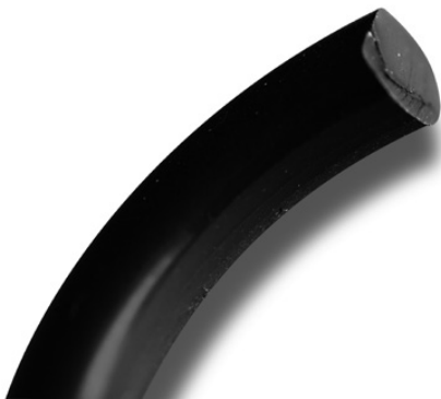
Fig. 10.12 Wear is seen as flattening of O-ring on one side
