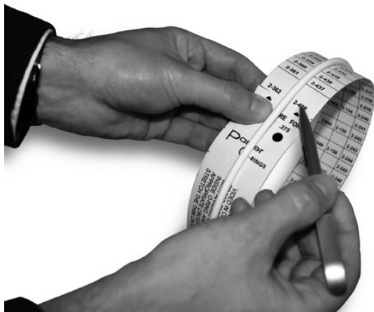
Fig. 5.9 Determination of the O-ring size using the measuring band
