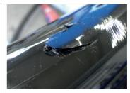
4.2 Melt the damaged area with the hot-air gun at approx. 600°C locally. Immediately when the material is melting, use a spoon or putty knife to press the melted material into the damaged area.
