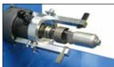
Simultaneous internal and external skiving. (USM 100)
