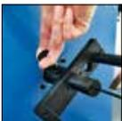
Easy exchange of skiving tool using a locking pin on USM 10 S.
