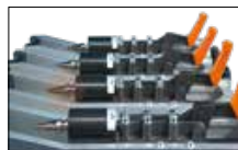
Axially adjustable quick-change system with adjustable rotating head.
