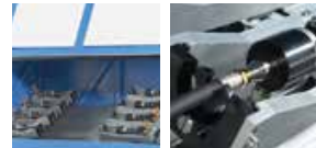
2 clamping discs per head, catering to various diameters (OD 8-42 mm). For hose assembly up to DN 19 (3/4"). Other sizes on demand.
