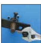
Blade adjustments for skiving depth need only to be made once for each hose dimension on the USM 10 S.
