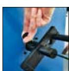
Easy exchange of skiving tool using a locking pin on USM 10 S.
