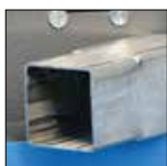
Special dies for forming tubes with square or round ends.
