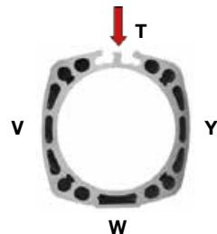
With 2 T slots on the top - FPM scraper, stainless steel end covers screws
