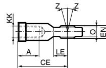
Use stainless steel nut with stainless steel swivel rod eye.
