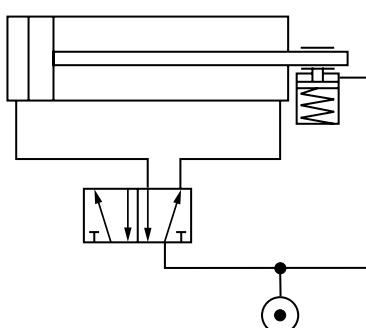
This solution is used to lock the cylinder in the event of a pressure loss in the system. A TEE piece is fitted in the pipe feeding the working valve for the cylinder. The lock on the cylinder is supplied from this TEE piece. In the event of a pressure loss, the lock is vented immediately and is applied.
