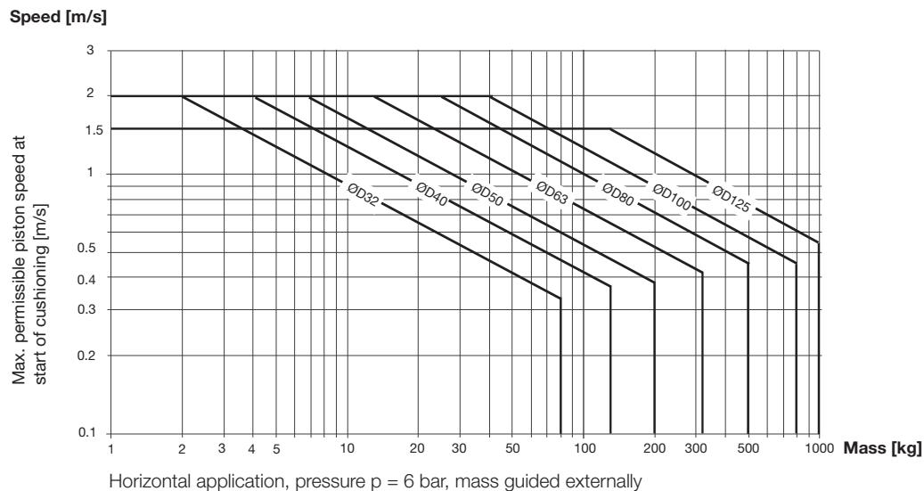
**Cushioning Diagram for Cylinders with rod locks**
