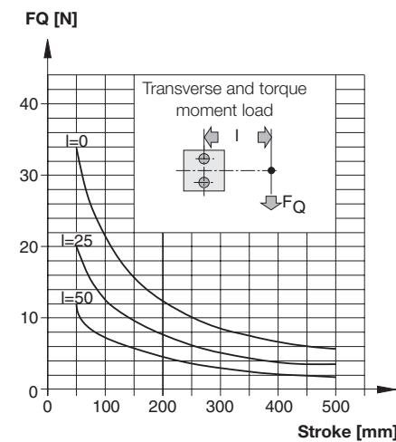
**Transverse and Torque Moment Load - Ø 40 mm**
