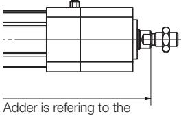
Adder is referring to the piston rod flat
