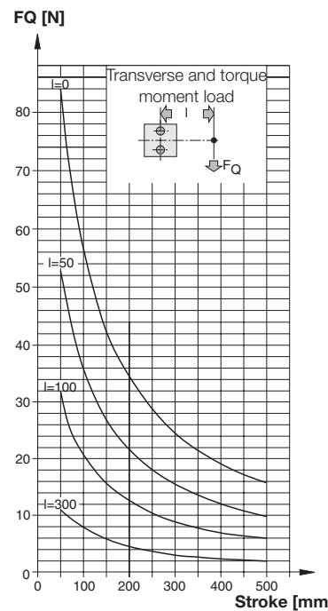
Transverse and Torque Moment Load - Ø 80 mm
