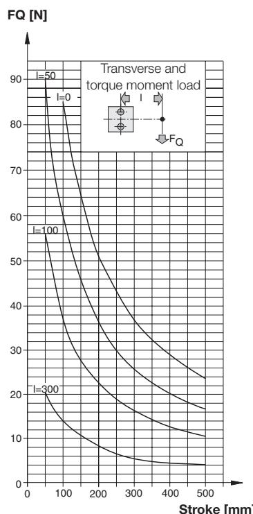
Transverse and Torque Moment Load - Ø 100 mm
