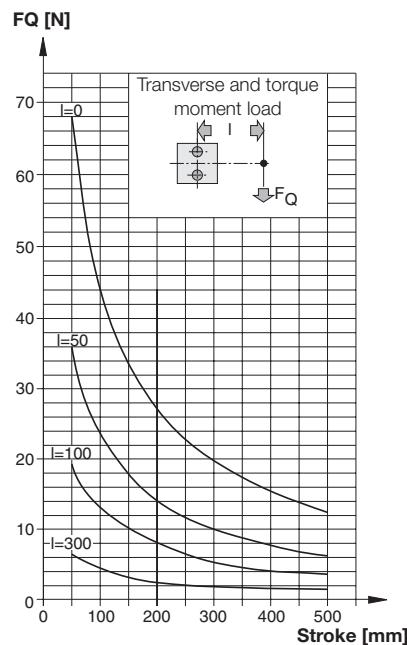
Transverse and Torque Moment Load - Ø 63 mm
