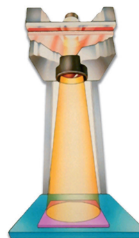
A focused light source is projected through a moving column of oil.
