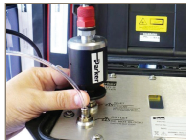
To remove the PRV, press down on the removal tool at the same time as lifting PRV off.
