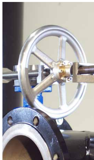
In large connection sizes the change-over is made with a hand wheel that operates two butterfly valves. Either valve is always open to ensure flow to the system.
