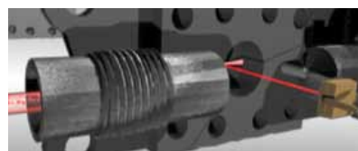
Fig 2. On reaching the photo diode cell, the highly accurate laser light is applied and projected through that oil column. The laser diode projects an image of the sample onto a photo diode cell.
