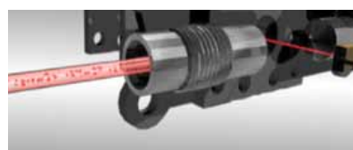
Fig 1. In simple terms a controlled column of contaminated fluid enters the laser optical scanner chamber. This design maintains contamination distribution within the fluid.
