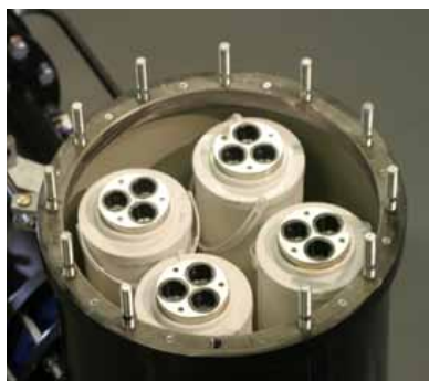
Filter vessels with multiple standardized elements. Bypass valves are fixed on the center tube inside the housing.
