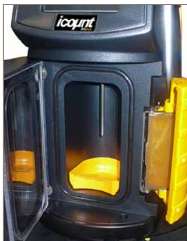
Fig 4. The IBSpplus oil sampling probe automatically lowers into the bottle once the test begins.
