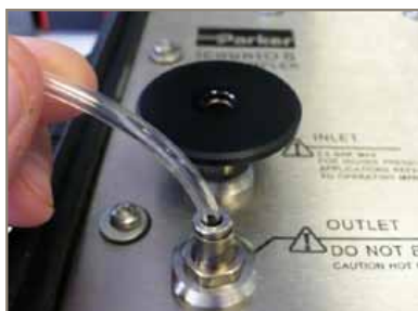
Attach OUTLET (Ø 4mm) hose
