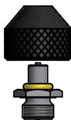
Model of valve stem 7/8" 14 UNF (B)
