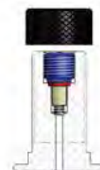
Model of valve stem integrated 5/8" 18 UNF (D)
