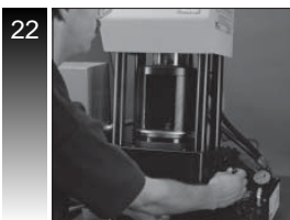
22 Crimp fitting onto hose until die ring contacts base plate.
