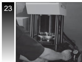
23 Push valve handle towards the rear to retract pusher and open die set.
