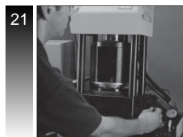
21 While holding hose and fitting in position on die step, lower pusher by pulling valve handle forward.
