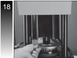
18 Insert front half of split die ring aligning pin in rear half with hole in front half.
