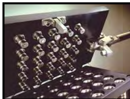
Hydraulic control circuit panel utilizing 1/8" HN style panel couplings and cam-locking device.
