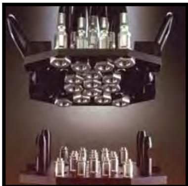
Typical hydraulic control circuit panel incorporating twelve 3/8" BN semi balanced couplings and three 1/2" BN semi balanced couplings (no additional separation force when pressurized). Two plate system utilizing cam-locking devices.
