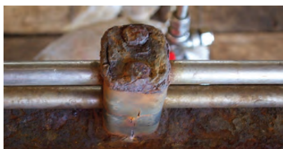
Crevice corrosion between the tube/tube trap interface.
