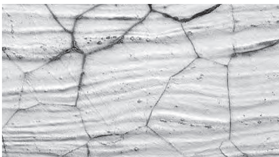
Intergranular Corrosion – HAZ Area – Stainless Steel Weld in Seawater Environment
