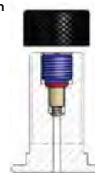
Model of valve stem integrated 5/8" 18 UNF (D)
