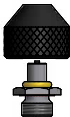
Model of valve stem 7/8" 14 UNF (B)
