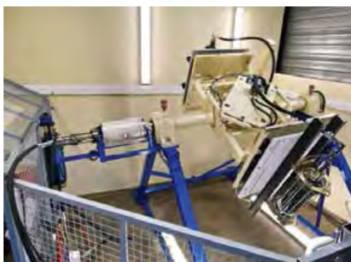
Accumulator test bench for wind turbine application.
