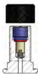
Model of valve stem integrated 7/8"14 UNF (C)
