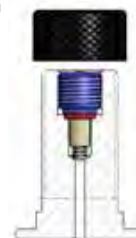
Model of valve stem integrated 5/8" 18 UNF (D)
