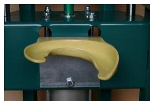
If you need to compress a coil spring, first make sure that you have selected the right equipment based on the information provided above. If you are fitting the strut at the bottom, first ensure that the diameter of the coil spring is larger than the internal lips on the selected spring holder. This is important to avoid the spring slipping under pressure.
