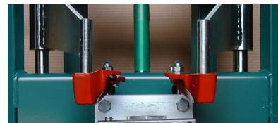
You may need to replace the standard spring holders with different holders. These could be spring holders with short lips (see the photo above) for vehicles manufactured in Japan by vendors such as Toyota and Honda. Other special spring holders are available for various vehicles.
