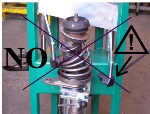
Use the press for pressing springs on McPherson struts only!
