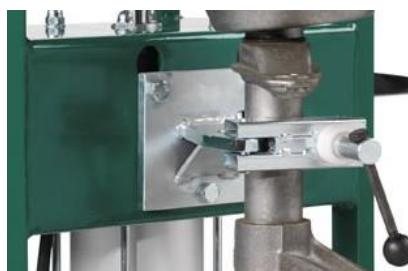
To make sure that the lips on both spring holders are correctly seated, pull the swivel arms outward by slowly building up down-pressure. If the spring holders can be pulled out, the lips are not clamping properly!!
