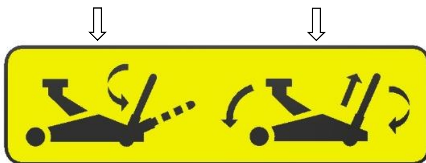
Change pull handle position, turn counter-clockwise
