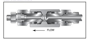
Dual-Disc Line Filters are utilized in numerous industrial, chemical processing, aerospace, nuclear and other applications. With the dual-disc design, large contaminant particles are trapped by the upstream filter element before they can reach and clog the smaller micron-size downstream element. Filter elements can be easily replaced.
