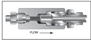
High Flow Cup-Type Line Filters are recommended in low pressure systems requiring both high flow rates and maximum filter surface area. Widely used in the industrial and chemical processing fields, the cup design offers as much as six times the effective filter area as compared to disc-type units. In addition, the filter elements can be quickly and easily replaced.
