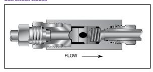
Minimum operating temperature for standard ball check valves 0°F (-17.8°C).
