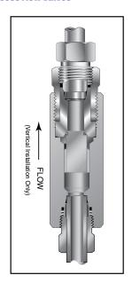
Protects pressure gauges and other pressure instrumentation from sudden surges in flow due to operator error or line failure. This valve provides dependable, tight shut-off.
