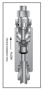
Protects pressure gauges and pressure instrumentation from sudden surges in flow or venting in the event of line failure.
