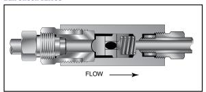
Minimum operating temperature for standard ball check valves -110°F (-79°C).
