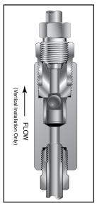
Protects pressure gauges and pressure instrumentation from surges in flow or sudden venting in the event of line failure.
