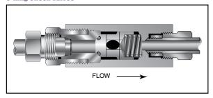
Minimum operating temperature for standard o-ring check valves 0°F (-17.8°C).
