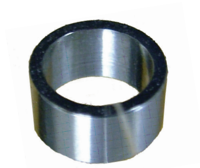
As-machined + Suparcase® Test Piece After Salt Fog Test
