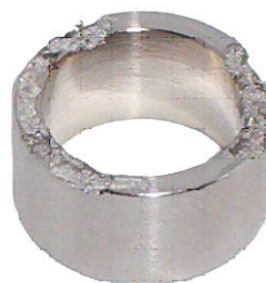
As-machined Test Piece After Ferric Chloride Test
