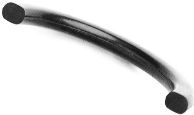
Fig. 10.8 Damage pattern caused by high compression set
