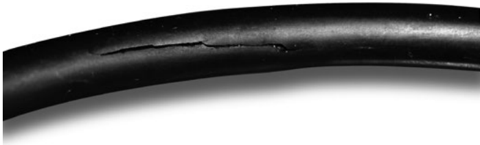
Fig. 10.11 O-Ring damaged by explosive decompression
