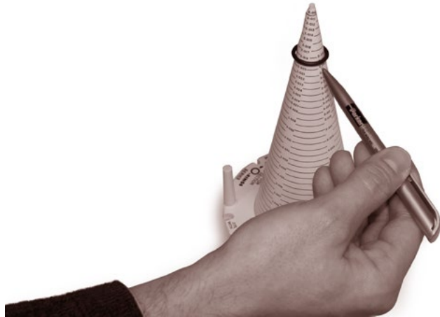
Fig. 5.4 Determination of the 2-xxx size number with the measuring cone
