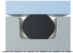
Fig. 10.1 Due to its elastic behaviour the O-ring exerts its sealing effect in the compressed, non-pressurised state between two sealing areas.
