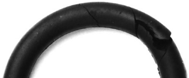
Fig. 10.10 Twisted O-Ring with cuts in surface
