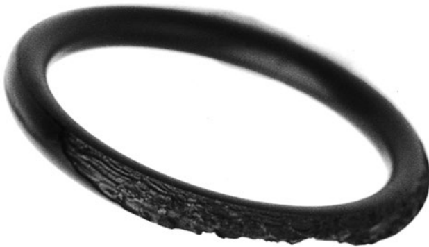
Fig. 10.6 Partially extruded O-Ring
