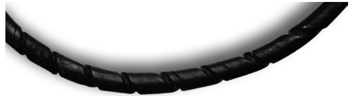
Fig. 10.9 Twisted O-Ring with spiral markings
