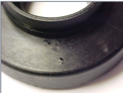
Burnt polymer pleat support mesh from arcing
